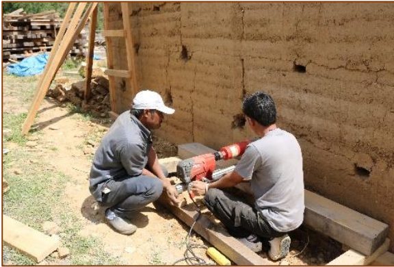
Coring of cylindrical specimens
