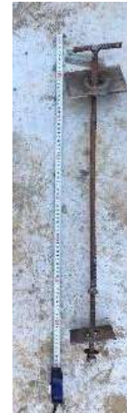
Figure 32. Threaded bar for outer & inner mesh connection
