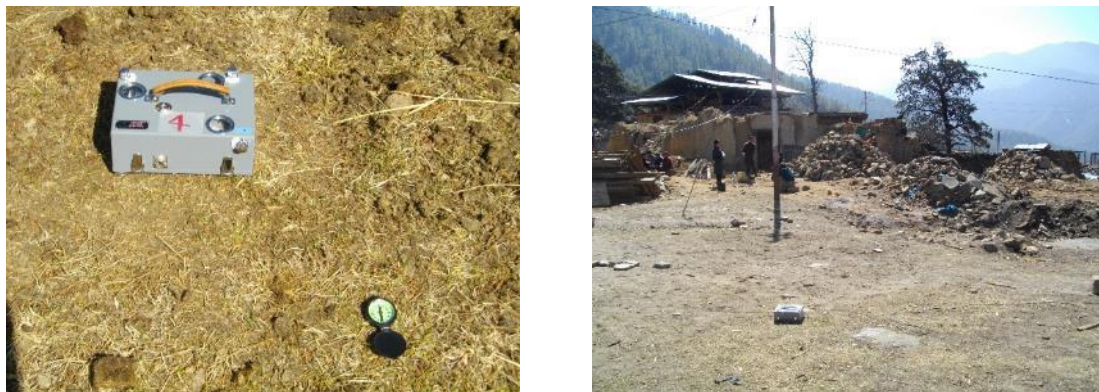
Figure 3-7. Microtremor measurement of ground at Tshenkher settlement of Talung village in the Haa Dzongkhag
