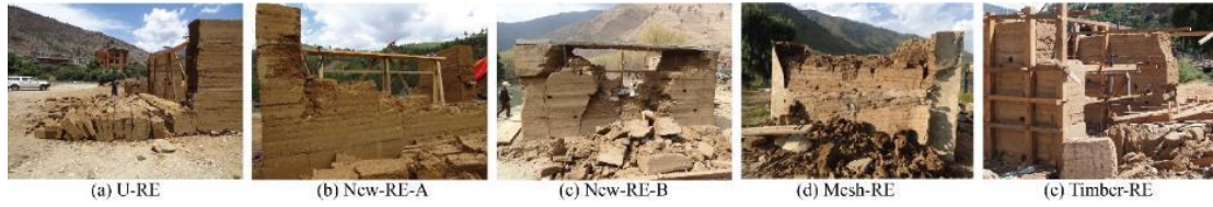
Figure 4-18. Final failure modes of all RE walls under out-of-plane loading
