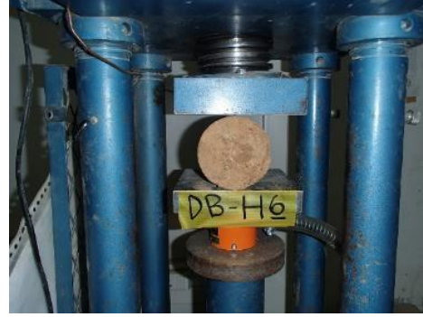
Figure 2-4. Tensile strength testing
