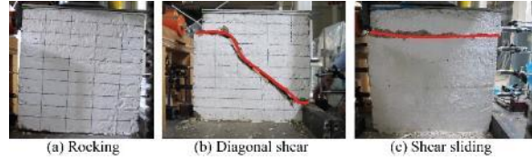
Figure 4-11. Typical failure patterns of RE wallettes observed under shear loading
