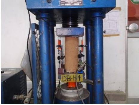
Figure 2-3. Compressive strength testing
