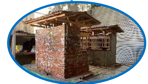
Shaking Table Test
