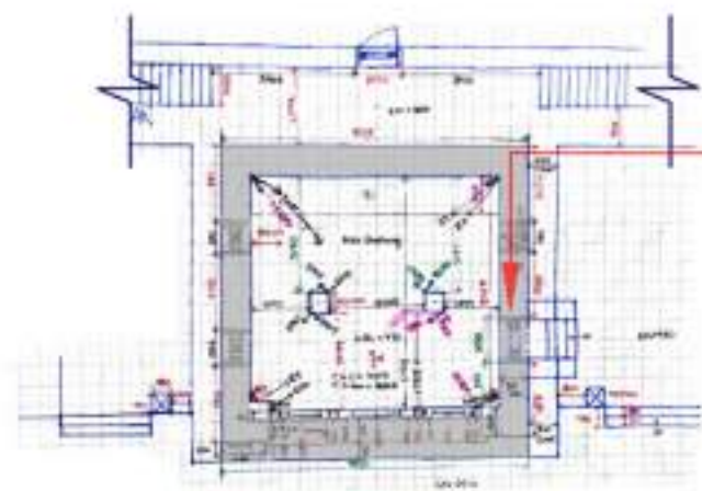
Layout of the plan is in the form of a giant mandala. Old structure of Könchogsum Lhakhang is constructed with thick stone masonry wall painted with lime on the outside.
